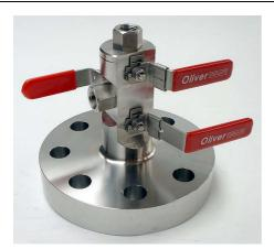
Machined from a single piece of 'grain flow controlled' forging, this valve features two inline ball pattern primary and secondary isolating valves and a heavy-duty ball vent valve.
