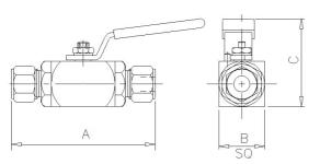
The 'B6' Type Single Isolating Ball Valve is designed for safe and reliable isolation giving bubble tight shut off. Totally enclosed soft seats offer both positive sealing and low operating torques, from vacuum to highpressure service. Anti-blow out spindle is fitted as standard with the option of PTFE or Grafoil seals.
