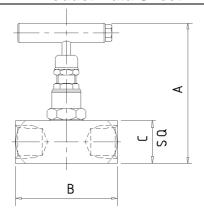
The 'F' Type Single Isolating Needle Valve is designed for safe and reliable isolation giving bubble tight shut off, non-rotating & anti-galling tip and dynamic self-adjusting spindle seal to give long service life in a variety of applications.
