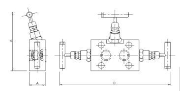
The 'Y34' and 'YV34' Type 3 valve manifolds are designed for direct mounting to differential pressure transmitters, with separate isolation for LP and HP inlets plus equalising valve for simple calibration. Each needle valve head is designed for safe and reliable isolation, giving bubble tight shut off, with non-rotating & antigalling tip and dynamic self-adjusting spindle seal to give long service life in a variety of service conditions.
